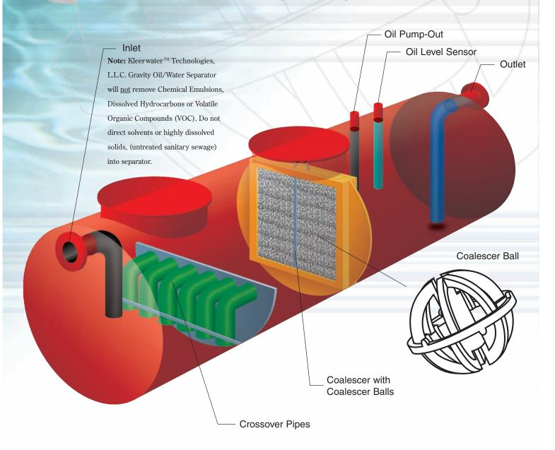
The development of the patented Coalescer "Ball" (U.S. Patent No. 5,229,015) by Kleerwater <sup>™</sup> is a technological breakthrough in the Oil/Water Separator industry. Its increased performance results in benefits and cost savings for you.
