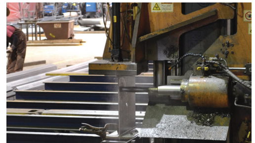
CNC Drill Line with 62' Bed. Drills Beams, Channels, Tubing, and Angles
