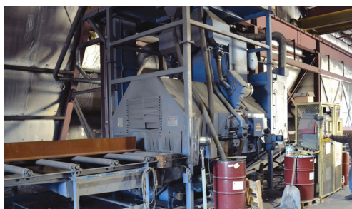
4 Wheel Shot Blaster with 6' Conveyor
