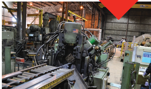
Angle Line can run up to .5"x6" FB and L6x6x.5 Cut and Punch
