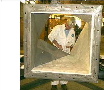
Chute with Ceramic Liner
