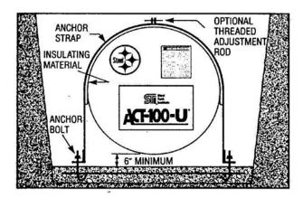
5.2 If a metallic hold-down strap is used, a pad of inert insulating dielectric material must be used to insulate the hold-down strap from the tank. The separating pad shall be wider than the holdsown straps, which will prevent direct contact between the straps and the tank shell. This pad is not required if the hold-down strap is fabricated from non-conductive material.
